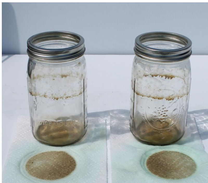
Figure 1. Fomesafen + paraquat with an incompatible non-ionic surfactant.
