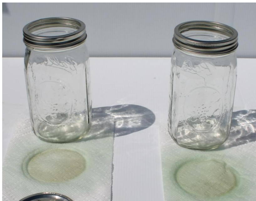
Figure 2. Fomesafen + paraquat with a compatible non-ionic surfactant.
